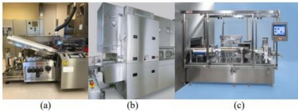
Gambar 3. 14 Rangkaian Mesin In Line dimana (a) Mesin Bosch RRU, (b) Mesin Bosch HQL, (c) Mesin Bosch ALF
